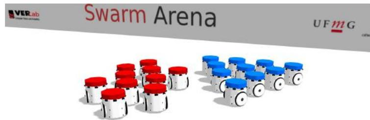
Figure 5.1: Flocking-segregative behavior. A swarm of heterogeneous robots demonstrates the ability to simultaneously exhibit segregation and flocking behaviors, relying solely on local sensing. The robots navigate a physically simulated environment containing obstacles, autonomously forming distinct groups while maintaining cohesive navigation through the terrain. This illustrates the concurrent manifestation of both segregation and flocking behaviors.
